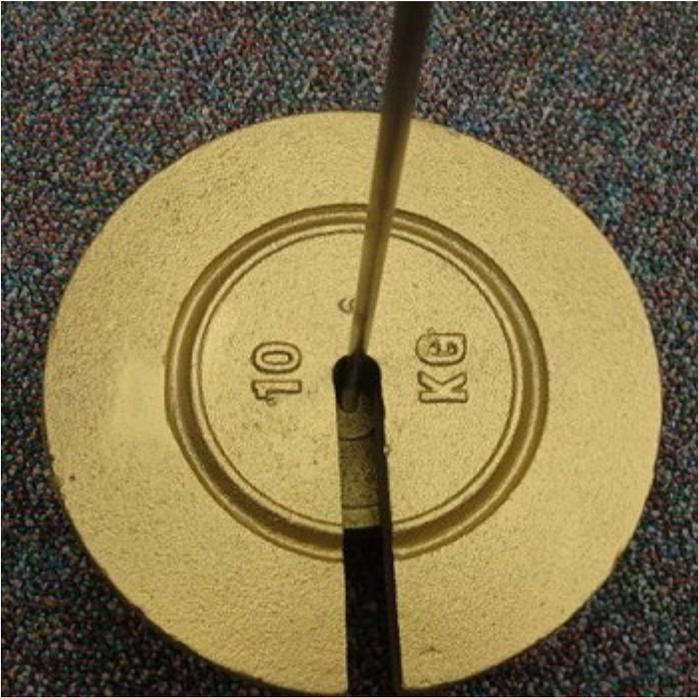
**Figure 6. Positioning the stem in the center of the weight's slot**
