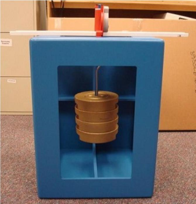
**Figure 7. Weights hanging from the dynamometer handle**
