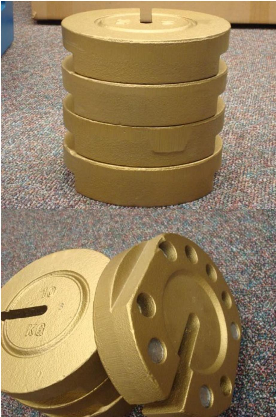
**Figure 5. Indentation in weights for lifting**
